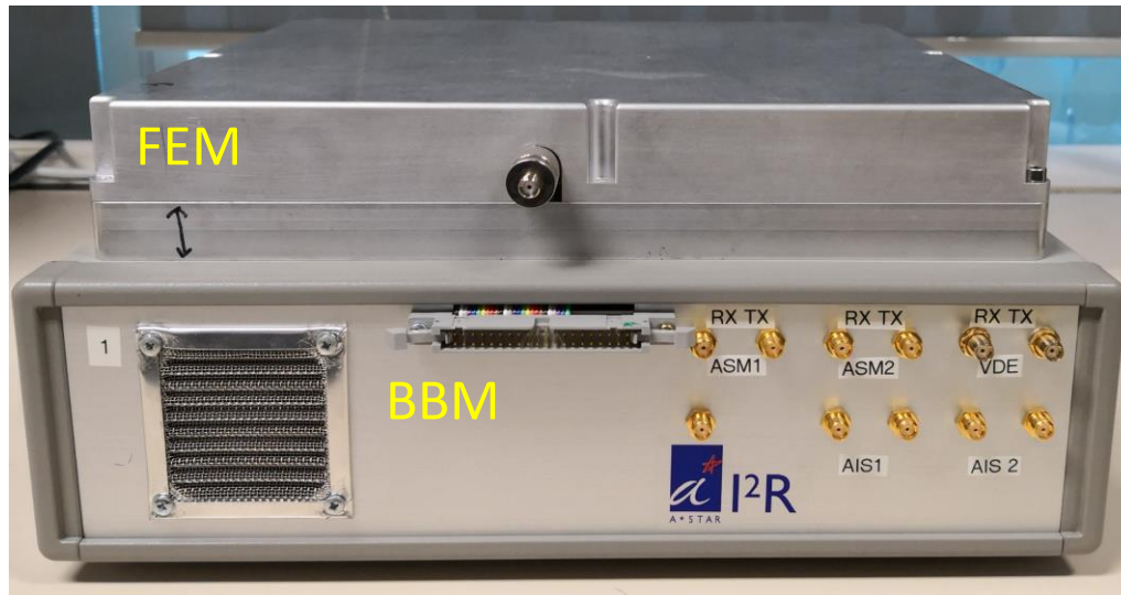
Figure 2. Ship-borne VDES Mobile Station - Final Prototype Hardware Version
